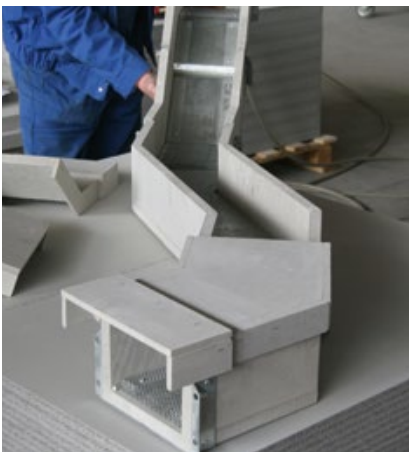
Duct elements and moulded parts are prefabricated to exact dimensions.
