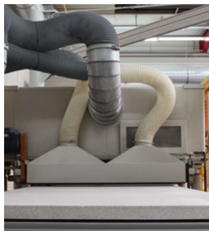
Aestuver® fire protection boards are first calibrated and the surfaces are sanded.
