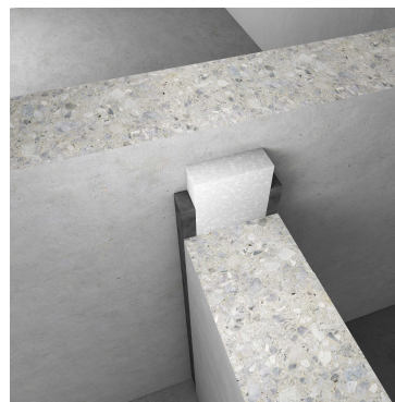
■ Aestuver™ FPM mastic double-sided with polystyrene as backfilling – option 2
