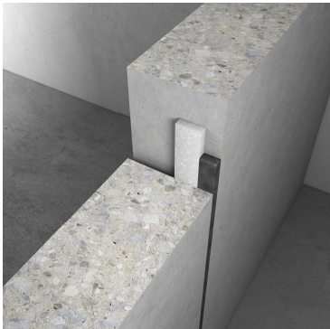
■ Aestuver™ FPM mastic single-sided with polystyrene as backfilling – option 1
