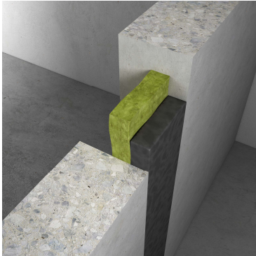
■ Aestuver™ FPM mastic single-sided with mineral wool as backfilling – option 1 also double-sided executable
